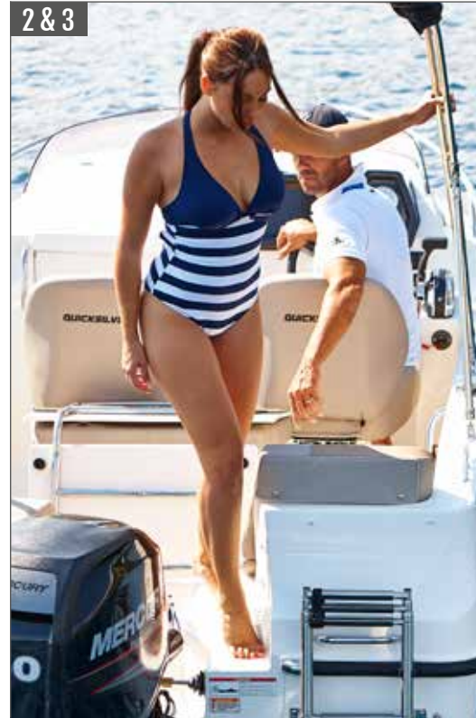
Bench seating flips up to allow boat access via the stern. Integrated step for boarding access
