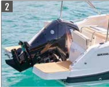
2 Reclining center backrest to allow full tilt engine position and maximal cockpit space
